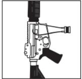
**BOLT ACTION RIFLES:** open the action or remove the bolt from the rifle. Then remove the magazine and insert the cable through the ejection port and out of the magazine well or the receiver assembly.
